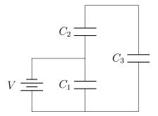
The circuit above contains 3 capacitors, all of initial value  $C = 4 \ \mu F$ . The voltage source is 10 V.
