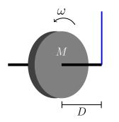
The angular momentum of the spinning disk is  $L = 124 \text{ kg-m}^2/\text{s}$ . The time it takes the gyroscope to make one complete revolution in the horizontal plane (its procession period) is 22.2 seconds.
