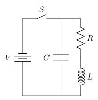
A circuit is composed of a battery with voltage V=10~V, one resistor  $R=75~\Omega$ , a capacitor C=20~pF, an inductor L=20~mH and a switch S. The switch has been open for a long time; at t=0, it is closed.
